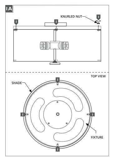
Install the shade by aligning the screws on the shade with the holes on the fixture and secure them together using the provided knurled nuts.
