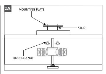
Remove the mounting plate from the fixture base by unscrewing the two knurled nuts from the two threaded studs.
