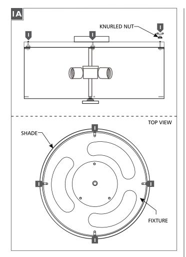
Install the shade by aligning the screws on the shade with the holes on the fixture and secure them together using the provided knurled nuts.
