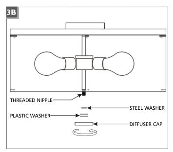
Unscrew the diffuser cap and remove it along with the washers from the socket assembly.
