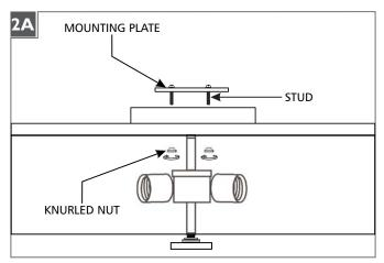
Remove the mounting plate from the fixture base by unscrewing the two knurled nuts from the two threaded studs.
