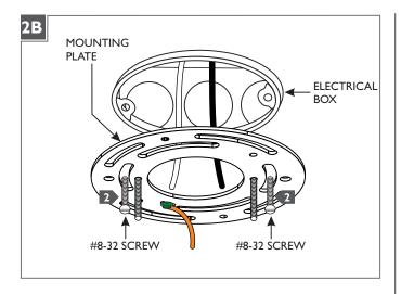
Mount the mounting plate to the electrical box with the two #8-32 screws.
