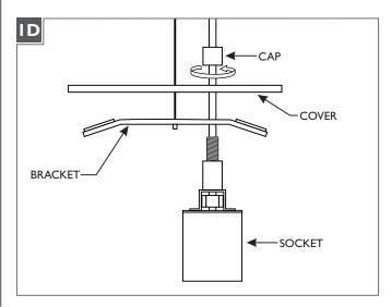
4 Disassemble the socket assembly by unscrewing the cap and separating the socket, bracket, and the cover.
