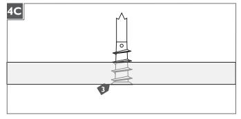
3 Screw the anchor in the rest of the way with a Phillips screwdriver.
