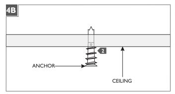
2 Tap the anchor at the marked point up to the threaded portion with a hammer.
