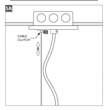
If necessary, adjust the aircraft cable until the fixture is level; feed the cable into the cable clutch to raise the fixture and push in on the cable clutch nipple to release the cable and lower the fixture.
