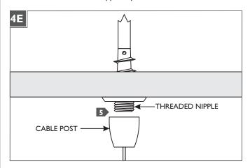
5 Screw the cable post completely to the threaded nipple.
