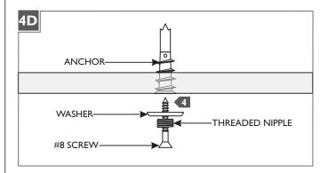
Insert the #8 screw into the threaded nipple and washer.
