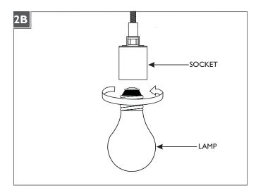
**CAUTION:** To reduce the risk of a burn or electric shock during relamping, disconnect the power to the fixture.
