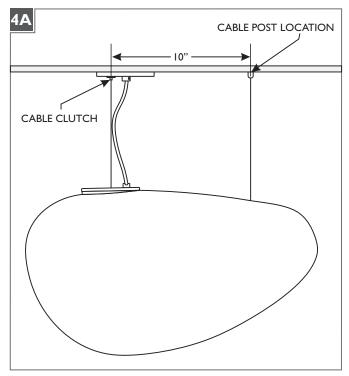
Mark the cable post location point 10" away from the center cable clutch on the canopy.
