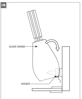
Carefully install the glass shade by aligning the opening on the glass shade to the slots on the socket and rotate downward at an angle that compliments the glass shade's curvature until it is firmly in place.
