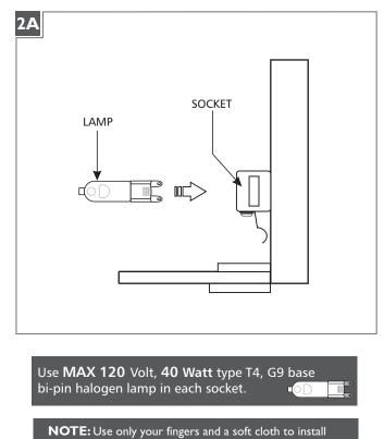
Push the lamp all the way into the socket. Repeat for remaining socket assemblies.
