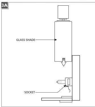
Carefully install the glass shade by aligning the opening on the shade to the slots on the socket and push it straight down onto the socket until it is firmly in place.
