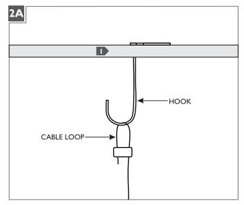
Install each crystal by placing the looped end of the cable onto each individual hook.
