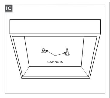
Mount the fixture base to the ceiling by installing it onto the mounting plate and securing it tightly with the two cap nuts.
