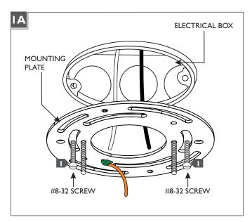
Mount the mounting plate to the electrical box with the two #8-32 screws.
