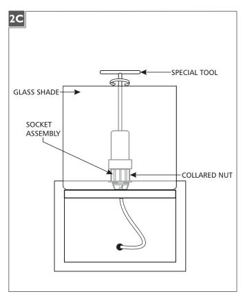
3 Secure the glass shade by re-installing the collared nut on the socket assembly and tighten it using the special tool.
