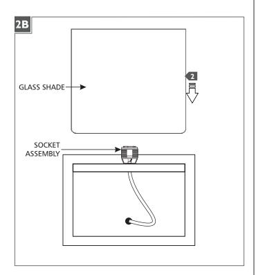
Install the glass shade by placing it on the socket assembly.
