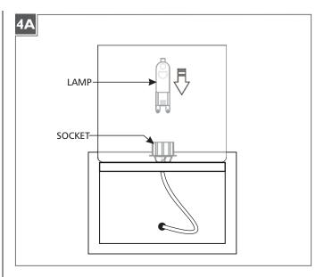
Use **MAX 120** Volt, **60 Watt** type T4, G9 base bi-pin halogen lamp.
