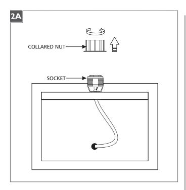
Unscrew the collared nut and remove it from the socket.
