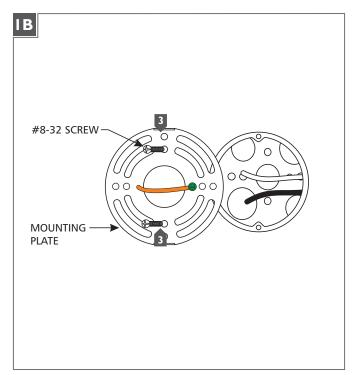
Install the mounting plate onto the electrical box with the two #8-32 screws provided.
