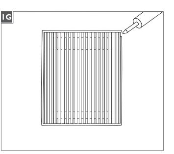
**I** For wet locations, caulk around the base with waterproof construction sealant.
