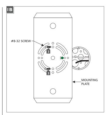
3 Attach the mounting plate to the electrical box using the two #8-32 screws provided.
