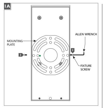
With the Allen wrench provided, remove the two fixture screws.
