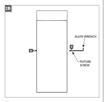
4 Remount the fixture onto the mounting plate and secure it tightly with the two fixture screws using the allen wrench.
