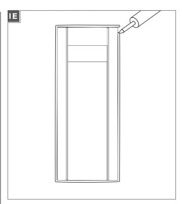
For wet locations, caulk around the base with waterproof construction sealant.
