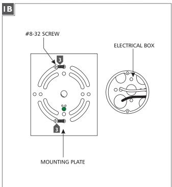
Attach the mounting plate to the electrical box using the two #8-32 screws provided.
