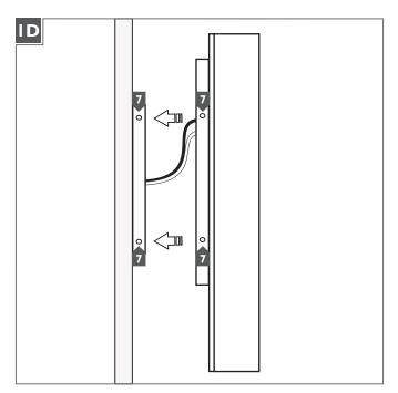
Reinstall the fixture onto the mounting plate and secure it in place with the four fixture screws.
