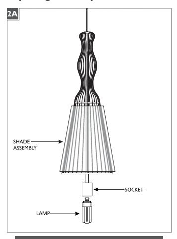
CAUTION: To reduce the risk of a burn or electric shock during relamping, disconnect the power to the fixture.
