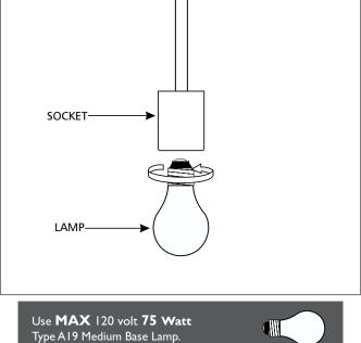
**I** Screw the new lamp into the socket.
