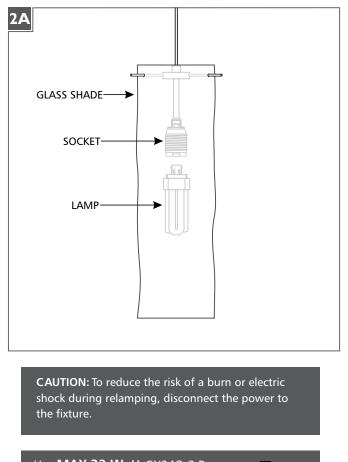
Use MAX 32 Watt GX24Q-3 Base Triple Tube Compact Fluorescent Lamp.
