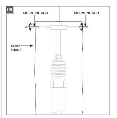
2 Place the hardware inside the glass shade and install the three mounting rods by screwing them in completely.
