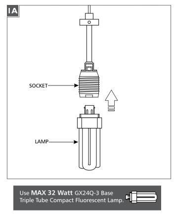
Push the lamp base into the socket.
