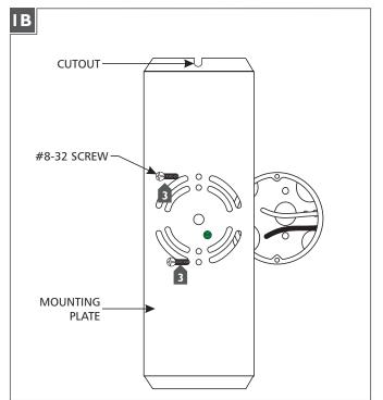
**Note:** When installing the mounting plate to the electrical box, be sure to have the cutout right side up.
