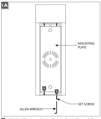
With the Allen wrench provided, back out (do not fully remove) the set screws at the bottom of the fixture.
