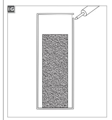
**I** For wet locations, caulk around the base with waterproof construction sealant.
