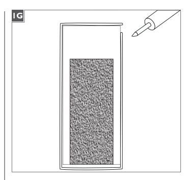
**I** For wet locations, caulk around the base with waterproof construction sealant.
