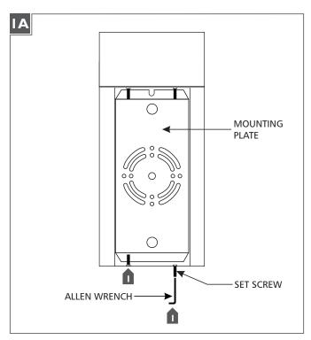
With the Allen wrench provided, back out (do not fully remove) the set screws at the bottom of the fixture.
