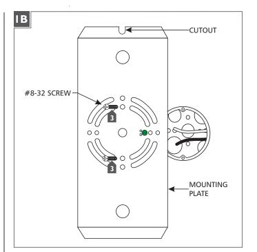
**Note:** When installing the mounting plate to the electrical box, be sure to have the cutout right side up.
