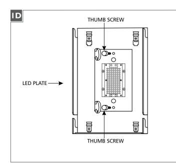
**7** Re-install the LED Plate and secure it tightly with the two thumb screws.
