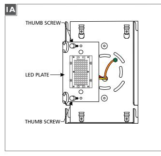
To gain access to the mounting plate holes, remove the two thumb screw to temporarily loosen the plate holding the LED lamp.
