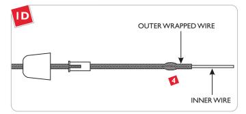
4 Slide the outer wrapped wire back to expose the inner wire.
