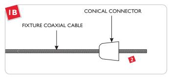
Insert the fixture coaxial cable through the conical connector.
