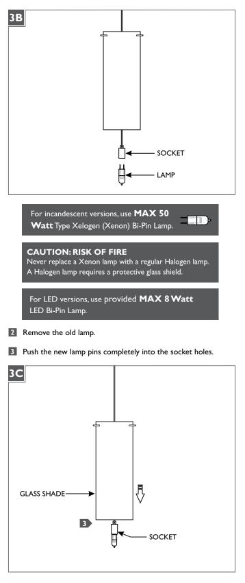
4 Lower the glass shade until the socket is properly inside the socket assembly.
