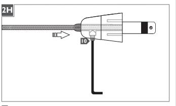
**IO** Firmly tighten the set screw on the conical connector.
