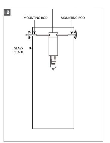
Place the hardware inside the glass shade and install the three mounting rods by screwing them in completely.
