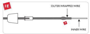
Slide the outer wrapped wire back to expose the inner wire.
