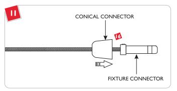
Slide the conical connector over the fixture connector. To install the fixture, refer to the instructions provided with the system.
