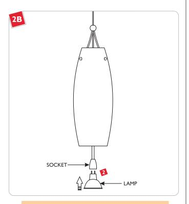
Use **MAX 50** Watt MR16 Front Cover Halogen Lamp.
