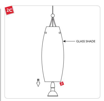
1 Lower the glass shade onto the socket assembly.
