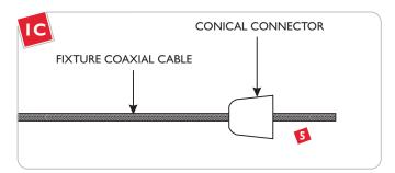
1 Insert the fixture coaxial cable through the conical connector.
