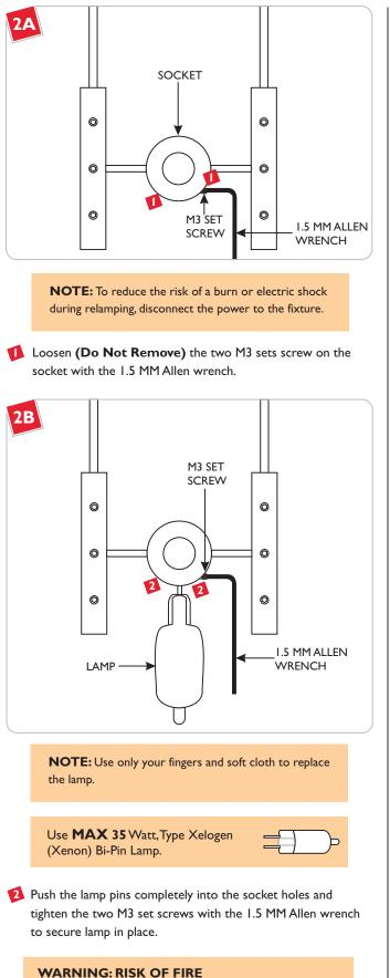
Never replace a Xenon (Xelogen) lamp with a regular Halogen lamp. A regular Halogen lamp requires a protective glass shield.
