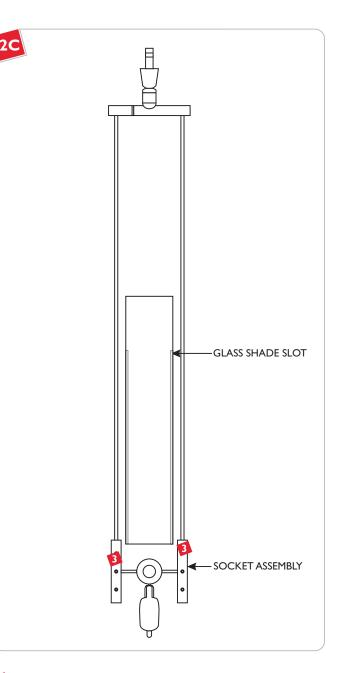
From between the fixture rods, carefully place the glass shade onto the socket assembly.
