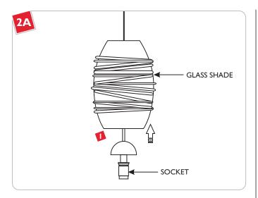
**NOTE:** To reduce the risk of a burn or electric shock during relamping, disconnect the power to the fixture.
