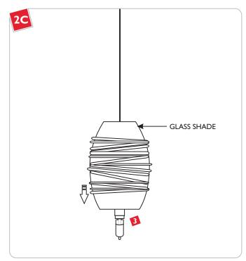
1 Lower the glass shade onto the socket assembly.
