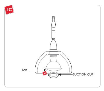
Remove the suction cup by pulling on the tab.
