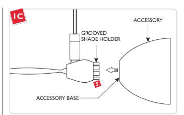
9 Push the accessory base onto the grooved shade holder.
