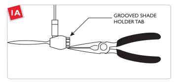
If the accessory fits tight onto the fixture, then carefully bend the grooved shade holder tabs in slightly with the needlenose pliers. If it fits loose, then carefully bend the grooved shade holder tabs out slightly with the needlenose pliers.
