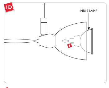
Push the lamp pins all the way into the socket holes.
