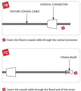
Insert the coaxial cable through the flared end of the stra relief.
