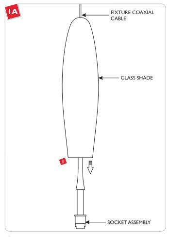
Feed the fixture coaxial cable through the glass shade. Slide the glass shade down the cord and rest it onto the socket assembly.
