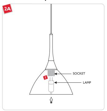
**NOTE:** To reduce the risk of a burn or electric shock during relamping, disconnect the power to the fixture.
