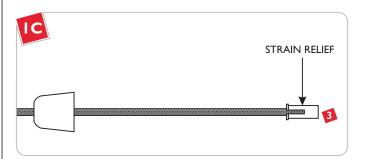
Insert the coaxial cable through the flared end of the strain relief.
