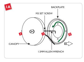
Loosen (Do Not Remove) the two M3 set screws on side of the canopy with the I.5MM Allen wrench provided.
