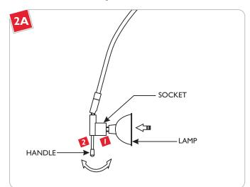
Use **MAX 50** Watt MR16 Front Cover Halogen Lamp.
