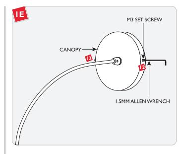
Place the fixture canopy onto the backplate. Level the fixture vertically and tighten the two M3 set screws with the 1.5MM Allen wrench to secure the fixture in place.
