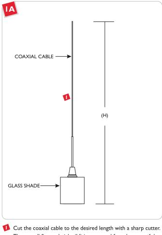
Cut the coaxial cable to the desired length with a sharp cutter. The overall fixture height (H) is measured from bottom of the glass shade to end of the coaxial cable.
