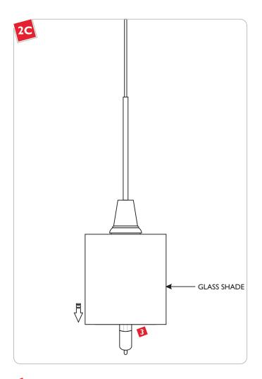
3 Lower the glass shade onto the socket assembly.
