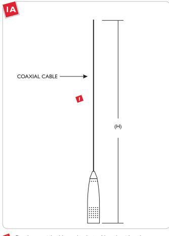
Cut the coaxial cable to the desired length with a sharp cutter. The overall fixture height (H) is measured from bottom of the Metal shade to end of the coaxial cable.
