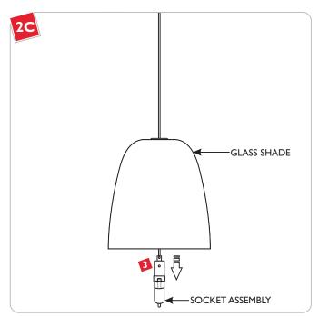
1 Lower the glass shade onto the socket assembly.
