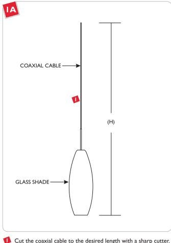
Cut the coaxial cable to the desired length with a sharp cutter. The overall fixture height (H) is measured from bottom of the glass shade to the end of the coaxial cable.
