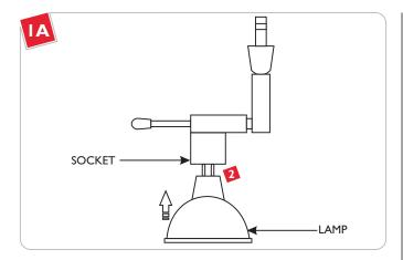
**NOTE:** To reduce the risk of a burn or electric shock during relamping, disconnect the power to the fixture.
