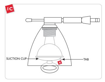
Remove the suction cup by pulling on the tab.
