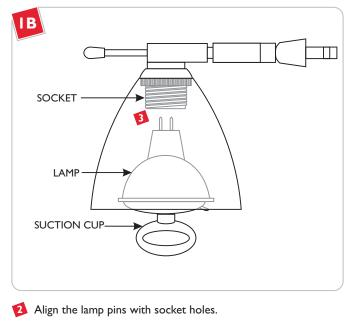
3 Push the lamp pins completely into the socket holes.
