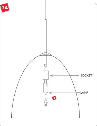
**NOTE:** To reduce the risk of a burn or electric shock during relamping, disconnect the power to the fixture.
