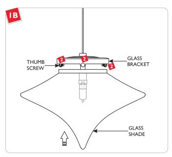
Place the glass shade completely into the glass bracket and tighten the three thumb screws to secure the glass shade in place.
