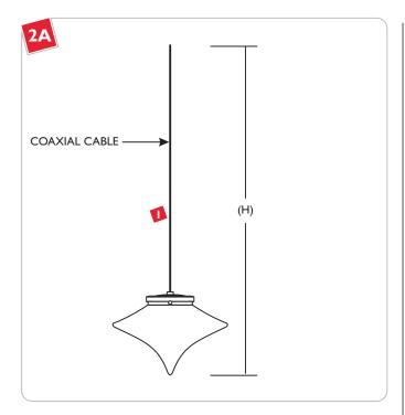
Cut the coaxial cable to the desired length with a sharp cutter. The overall fixture height (H) is measured from bottom of the glass shade to end of the coaxial cable.
