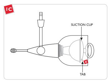
Remove the suction cup by pulling on the tab.
