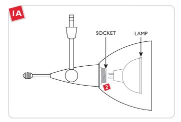
**NOTE:** To reduce the risk of a burn or electric shock during relamping, disconnect the power to the fixture.
