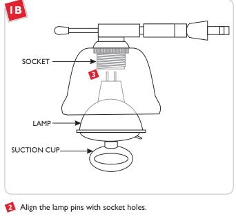
13 Push the lamp pins completely into the socket holes.
