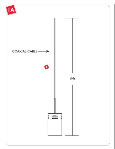
Cut the coaxial cable to the desired length with a sharp cutter. The overall fixture height (H) is measured from bottom of the metal shade to end of the coaxial cable.
