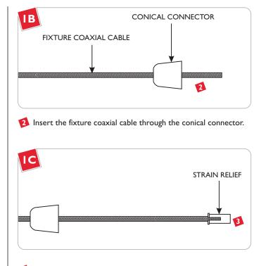
Insert the coaxial cable through the flared end of the strain relief.
