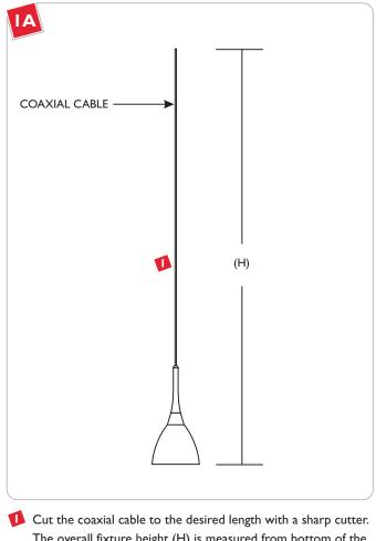
The overall fixture height (H) is measured from bottom of the glass shade to end of the coaxial cable.
