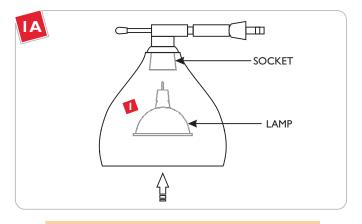
**NOTE:** To reduce the risk of a burn or electric shock during relamping, disconnect the power to the fixture.
