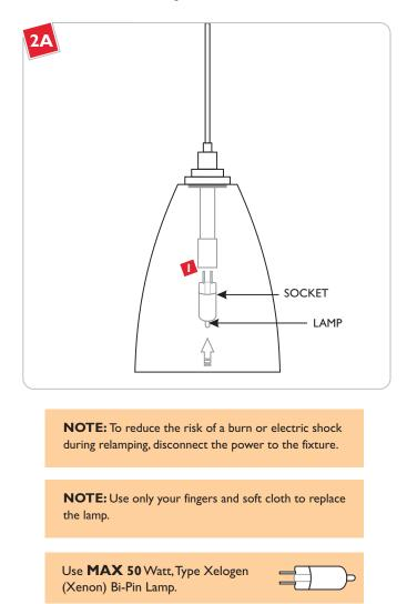
Push the lamp pins completely into the socket holes.
