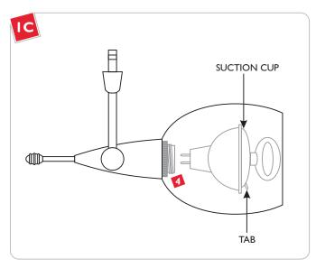
4 Remove the suction cup by pulling on the tab.
