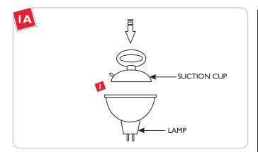
**NOTE:** To reduce the risk of a burn or electric shock during relamping, disconnect the power to the fixture.
