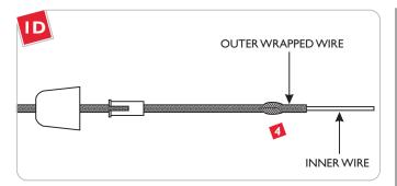
Slide the outer wrapped wire back to expose the inner wire.
