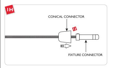
Slide the conical connector over the fixture connector. To install the fixture, refer to the instructions provided with the system.
