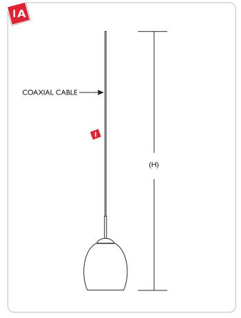
Cut the coaxial cable to the desired length with a sharp cutter.
