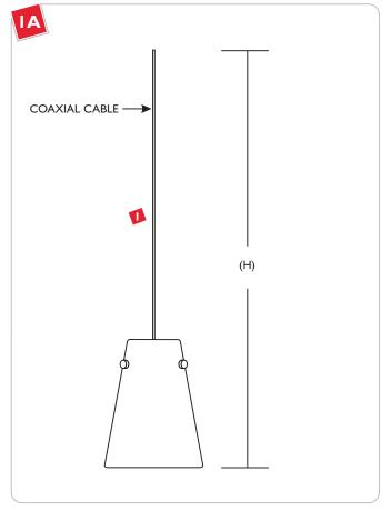
Cut the coaxial cable to the desired length with a sharp cutter. The overall fixture height (H) is measured from bottom of the glass shade to end of the coaxial cable.
