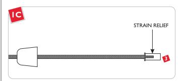
3 Insert the coaxial cable through the flared end of the strain relief.
