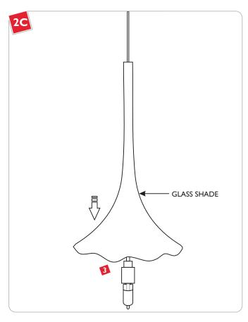
1 Lower the glass shade onto the socket assembly.
