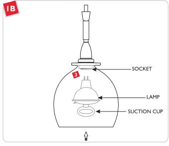
2 Align the lamp pins with the socket holes.
