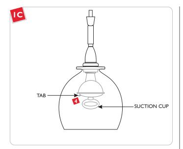
Remove the suction cup by pulling on the tab.
