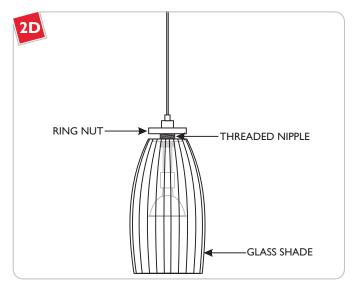
1 Lower the glass shade onto the socket assembly and tighten the ring nut to the socket assembly threaded nipple.
