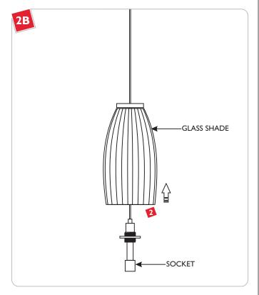
2 Lift the glass shade up to expose the socket.
