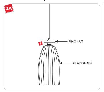
**NOTE:** To reduce the risk of a burn or electric shock during relamping, disconnect the power the fixture.
