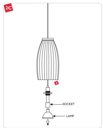
Use MAX 50 Watt MR16 Front Cover Halogen Lamp.
