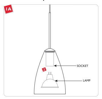
**NOTE:** To reduce the risk of a burn or electric shock during relamping, disconnect the power to the fixture.
