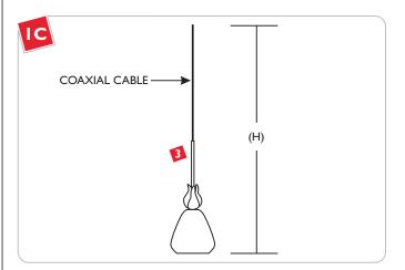
Cut the coaxial cable to the desired length with a sharp cutter. The overall fixture height (H) is measured from bottom of the glass shade to the end of the coaxial cable.
