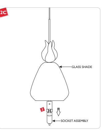
3 Lower the glass shade onto the socket assembly.
