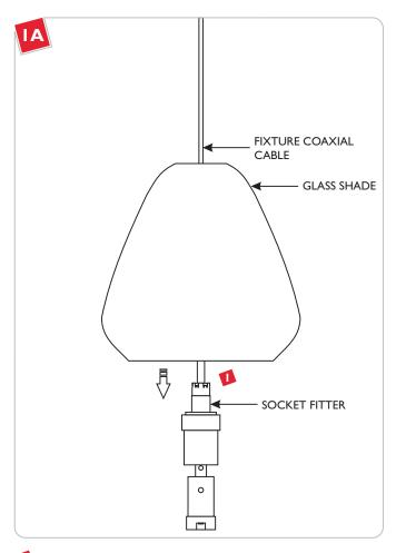
Feed the fixture coaxial cable through the socket fitter and glass shade. Slide the glass shade down the cord and rest it onto the socket fitter.
