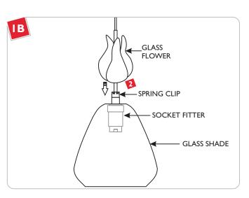
2 While holding the socket fitter against the glass shade push the glass flower completely onto the socket fitter spring clip.
